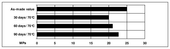
Lap shear strength versus temperature (ISO 4587) (typical average values)
