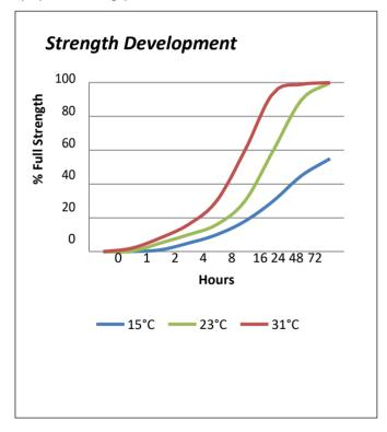
Graph shows typical strength development of bonded components. An increase of 8°C in temperature will halve the cure time. Lower temperatures will result in a slower cure time.
